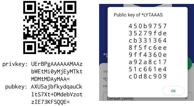
Figure 8: Attack 2 in practice: on the left, a suitable keypair (base64 encoded). The public key bytes 1 to 31, also encoded in the QR code, all consist of printable UTF-8 characters. On the right, the *LYTAAAS Threema gateway account (since revoked), with the hijacked public key of the server. User \mathcal{U} sending the contents of the QR to *LYTAAAS as a message will allow *LYTAAAS to authenticate to Threema as \mathcal{U} .
